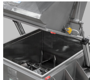
Dual pneumatic cylinders for opening cover
