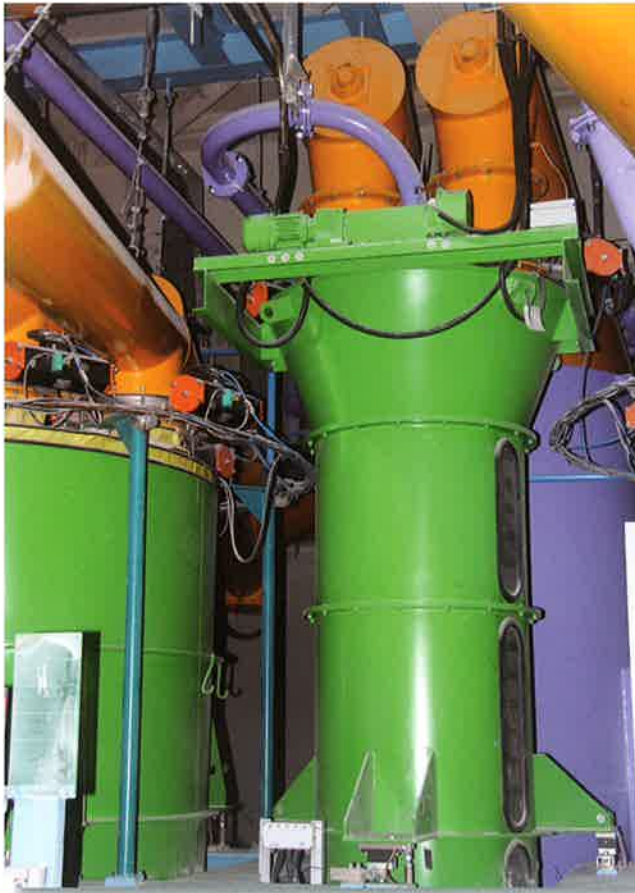
Figure 7: Volumetric measuring unit for lightweight aggregates
