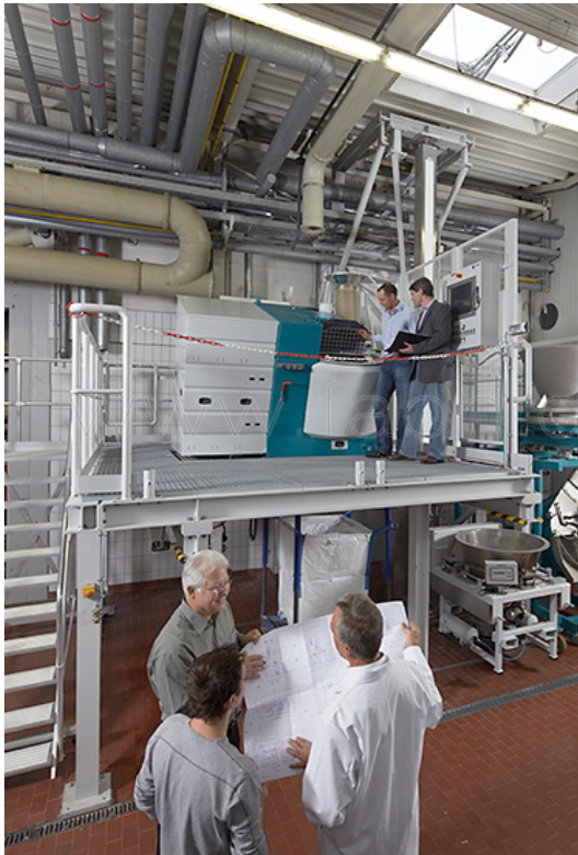
Fig 12: Eirich preparation plant for graphite specialties
