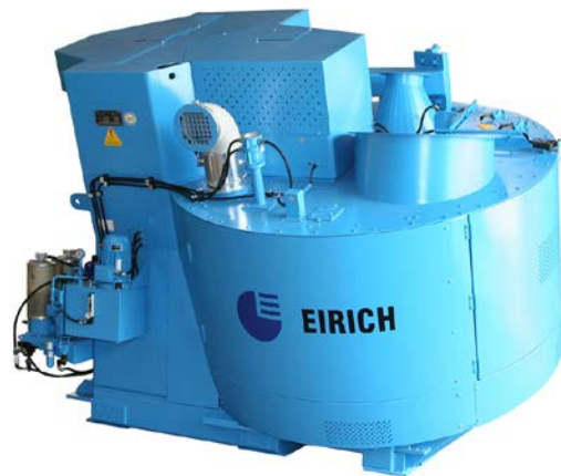
Fig 2: RV 24 conti remixer-cooler for a Chinese anode plant
