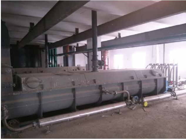
Fig 8: Coke screw heater 2 x 32 t/h
